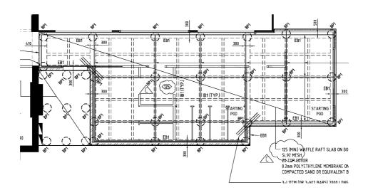
Photo 1: Slab & footing plan showing layout grid of the waffle pods
